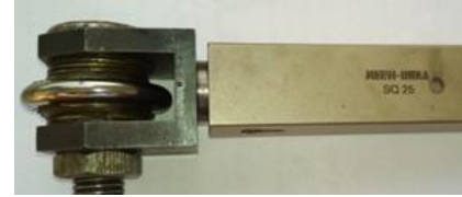
Fig.2. (a) Photographic view of roller burnishing tool [25]
