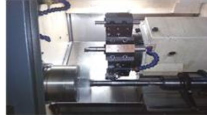
Fig.2 (b) Experiment setup of roller burnishing process [25]
