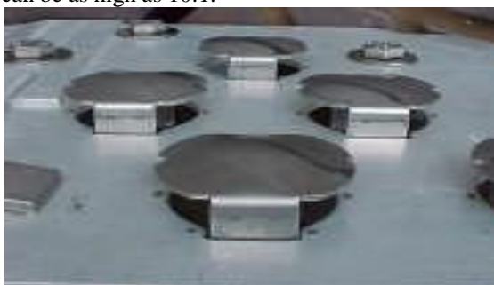
Figure 4. Schematic of Valve Trays
