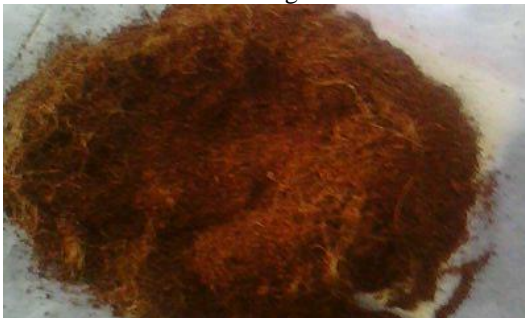
Fig No.2 Coconut husk particles after screened through IS Sieve-300micron and retained on IS Sieve-150micron
