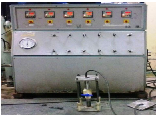
Figure Error! No sequence specified. Test setup for testing of ball valve
