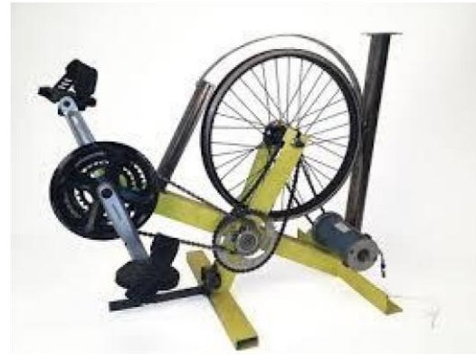
Fig 2: Chain Drive in Bicycle Generator
