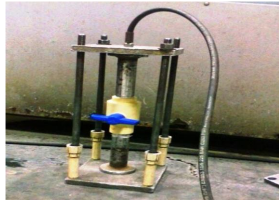
Figure 2 Fixture arrangement for testing of valve.
