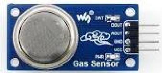
Figure: 3.8 MQ-135 Gas Sensor
