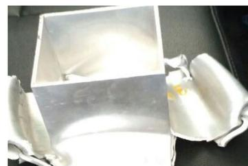
Fig 1.11 Failed compression sample
