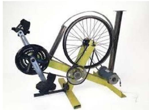
Fig2: Chain Drive in Bicycle Generator
