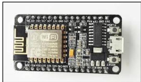
Figure 3.6:- Node MCU Wi-Fi Module
