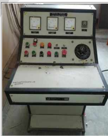
50 Kv AC & 70 Kv DC Voltage Test Setup
