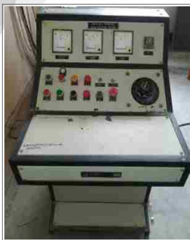
50 Kv AC & 70 Kv DC Voltage Test Setup
