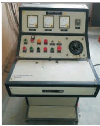
50 Kv AC & 70 Kv DC Voltage Test Setup
